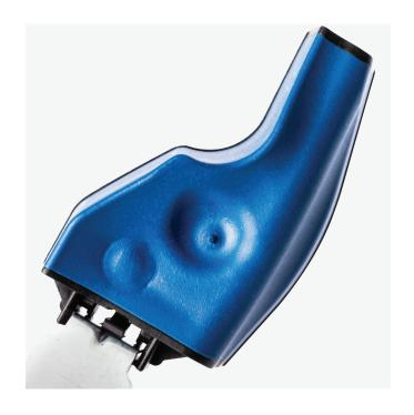
Composite Body Solutions (CBS™) for closures helps to improve the performance, stiffness, fatigue, NVH, and lightweighting. The structural adhesive distributes the loads better than traditional welding. The CBS™ part is able to bond to all four walls of the cavity, to take advantage of the entire section.
