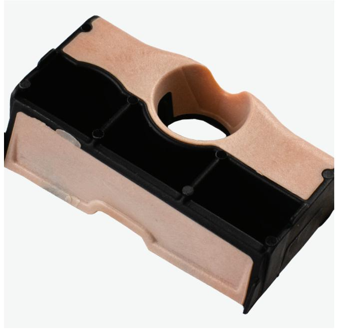
Composite Body Solutions (CBS™) are used as local mount reinforcements. Small CBS™ parts can be used to improve local body stiffness where point loads are applied and result in a high stress concentration.
