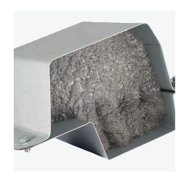
L&L's well-established portfolio of multiple heat activated foamable acoustic sealants are formulated to produce specific levels of volumetric expansion, density, and cell structure per formulation. They are designed to seal a gap between two substrates to prevent intrusion of air, water, dust, fumes, etc. Our acoustic sealants bond and protect surfaces to prevent corrosion to bare metallic substrates.
