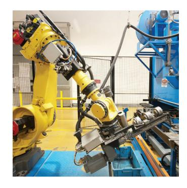
L&L Products' robotically extruded sealants technology combines our custom formulated chemistry with the capability of a fully automated application process. It involves extruding and applying an L&L formulation directly to a metal substrate by a robot.
