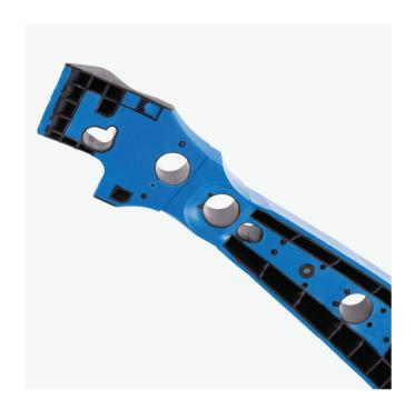
B-Pillar structural inserts are heat activated expanding adhesives with engineered carrier filled cavities. This bonds individual load bearing members to create a unified macro structure with significantly improved stiffness and strength attributes.
