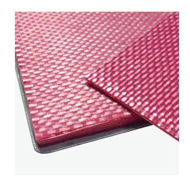
L&L Products Composite Panel Stiffener is designed to provide improved local reinforcement and NVH; specifically to deal with excessive panel vibration and noise issues. It comprises a high expanding structural adhesive contained within a fiberglass reinforcement.
