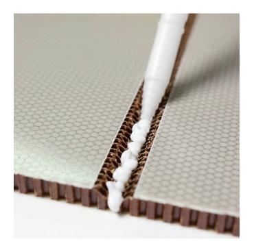
L&L Products develops FST compliant adhesives that introduce a new approach to bonding sandwich panels in aerospace applications.
