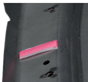
Tapes are applied prior to the E-coat oven.
