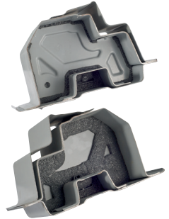
During the E-coat bake cycle, the sealant material expands to fill and seal the cavity.
