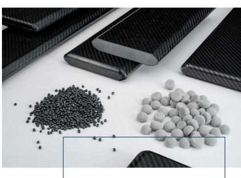
INSITUCORE® FOAMING CORE TECHNOLOGY IS A FAMILY OF ONE-COMPONENT HEAT ACTIVATED MATERIAL USED TO CREATE COMPOSITES WITH FOAM CORE.
