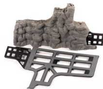
The sealant material foams and cures in the E-coat oven.
