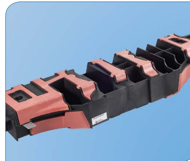
L&L Reinforce heat-cured CBS parts are specifically engineered for each automotive application. CBS can improve body stiffness, reduce noise, enhance crash performance and reduce weight by allowing the use of thinner gauge metals.
