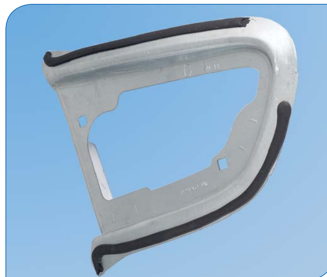
L&L XiP is a robotized application process for the custom-formulated materials from L&L's Acoustic, Seal or Bond product ranges. After extrusion directly onto the metal part, the materials are dry-to-touch and solid, eliminating wash-out problems.
